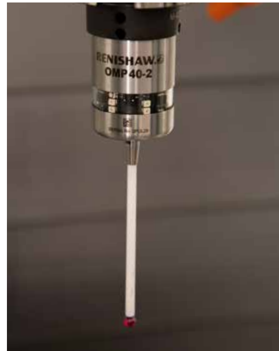
Part probes for quick, accurate set ups loads the tool data directly into the Tool Table.
