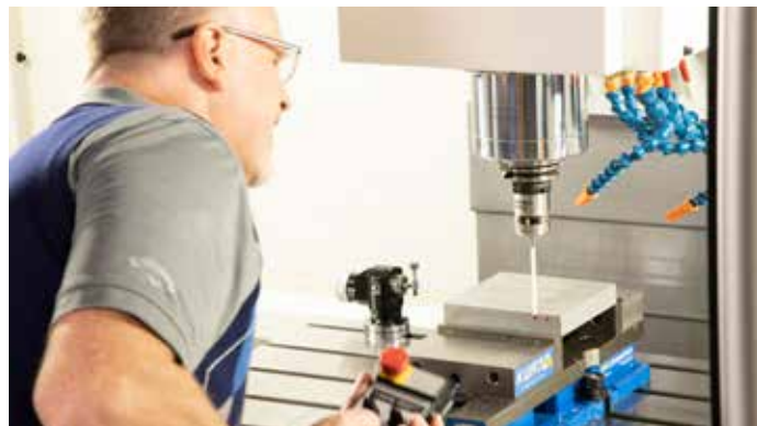
Part Measurement routines for part alignments in set-up and in-process measurement to check part dimensions.
