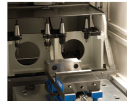
Internal: 8-station tool changer; X, Y, Z travels of 14" x 12" x 17"
