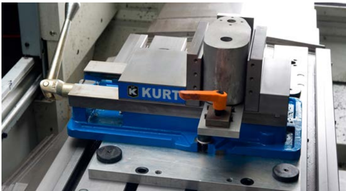
Fixture plate with integrated vice for quick setups.
