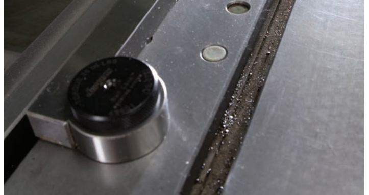
Optional Locating Guide Assembly allows you to easily reference your own features.
