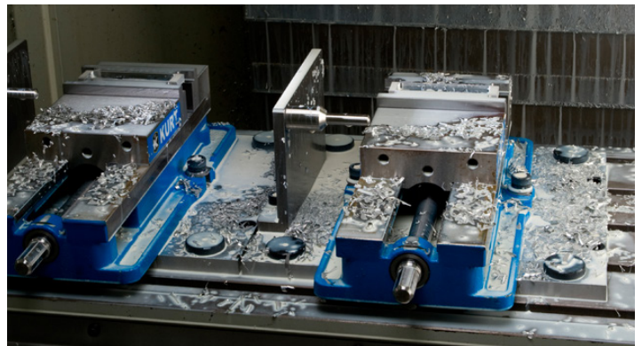
Fence and precision standoffs for quick, repeatable changes.
