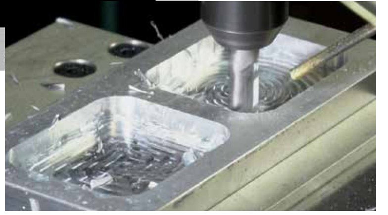
The pocket on the left has a standard tool path. The pocket on the right was machined with Adaptive tool path.
