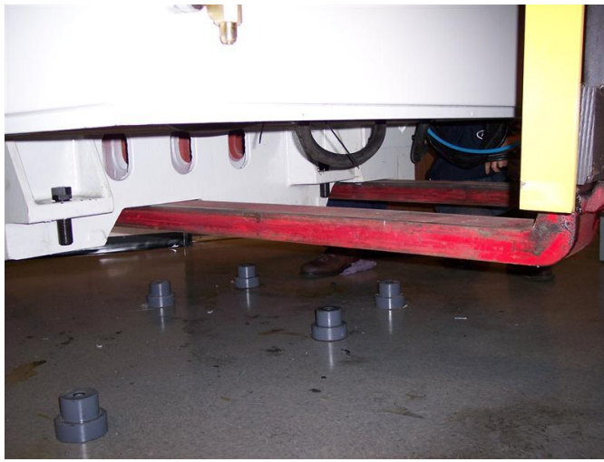
Figure 5 – Lifting the LPM
