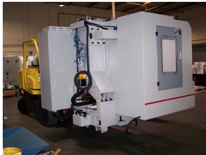
Figure 4 – Lifting the LPM
