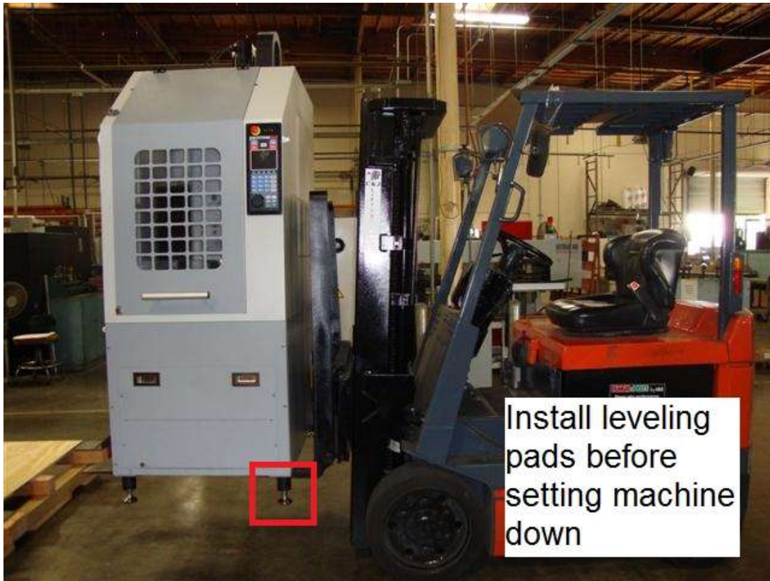
Figure 3 – Installing Leveling Pads
