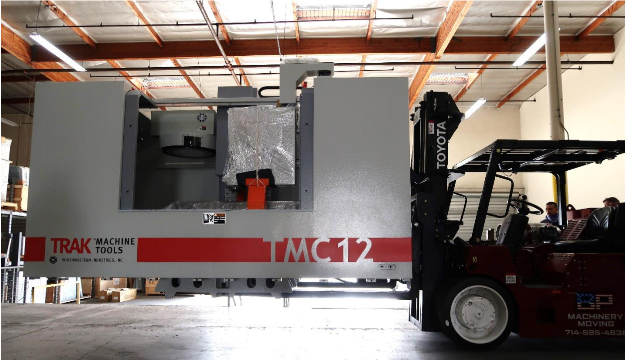
Figure 4 – Lifting the TMC
