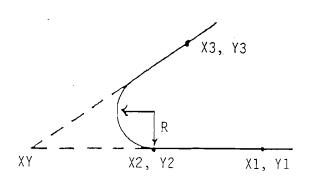
NOTE: Point X2,Y2 is on line X1, Y1--X2, Y2 and on the arc with radius R between the lines
