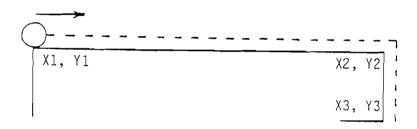
If the cutter in the sketch above is moving from left to right from point X1, Y1 to X2, Y2 and on to X3, Y3 then these actual points can be programmed instead of the center of the cutter.
