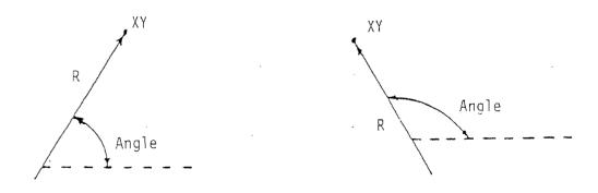
Display Prompts: RADIUS, ANGLE (NOTE: The angle is always measured from positive X axis or 3 o'clock.)
