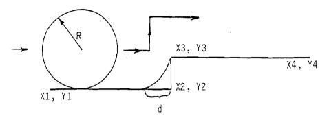
In the figure above, to mill from X1, Y1 to X2, Y2 to X3, Y3 to X4, Y4 when the length of the step from X2, Y2 to X3, Y3 is less than the radius (R) of the tool, point X2, Y2 would have to be offset toward point X1, Y1 by a distance equal to d. d can be calculated using the following formula:
