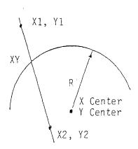
Display Prompts: X1, Y1, X2, Y2, XCENTR, YCENTR, RADIUS Number of possible solutions: 2, A and B
