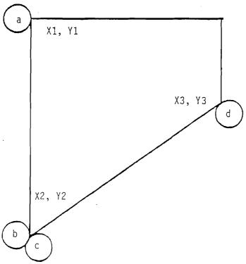
In the figure above if a DO ONE mill event was programmed from X1, Y1 to X2, Y2 with tool right offset the cutter would move from a to b. If another DO ONE mill event was programmed from X2, Y2 to X3, Y3 with tool right offset the cutter would first move from b to c (the end of the first to the beginning of the second with their offsets) then on command from c to d. Note that if the cutter is not raised in moving from b to c the tip of the corner at X2, Y2 will be machined off.
