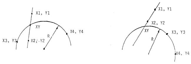
Display Prompts: X1, Y1, X2, Y2, X3, Y3, X4, Y4, RADIUS Number of possible solutions: 4; A, B, C, D
