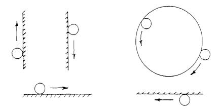
Tool center means no compensation either right or left. That is, the centerline of the tool will be moved to the programmed points.
