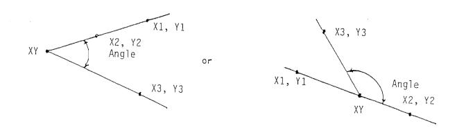
Display prompts: X1, Y1, X2, Y2, X3, Y3, ANGLE Number of possible solutions: 2, A and B
