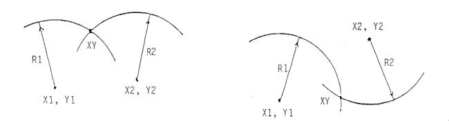
Display Prompts: X1, Y1, R1, X2, Y2, R2 Number of possible solutions: 2; A and B If only one solution is given the circles are tangent.
