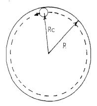
Or for the sketch above the actual desired circle with radius R can be programmed instead of the radius of the center at the cutter Rc.
