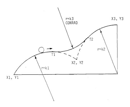
NOTE: CONRAD must always be the same or larger than the tool radius for inside corners. If CONRAD is less than the tool radius and an inside corner is machined, the ProtoTRAK will ignore the CONRAD.
