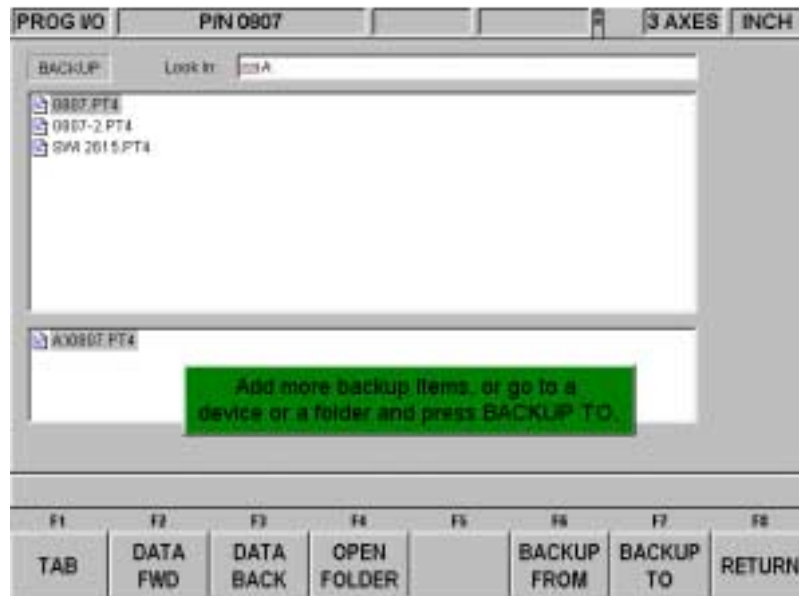
FIGURE 13.8 Backing up. The top part of the screen shows all the items in Drive A. The bottom part shows the items that have been picked for backing up
