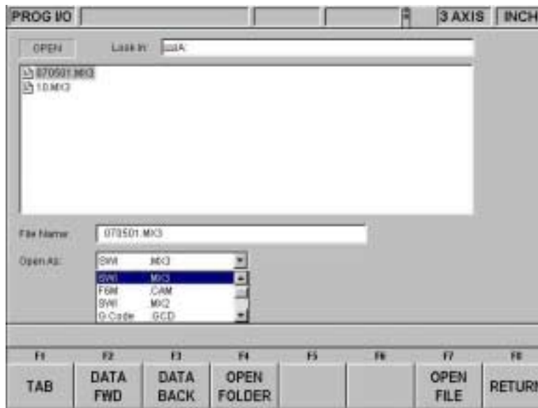
FIGURE 13.9.2 Use the Open As box to tell the ProtoTRAK SM CNC what kind of file it is
