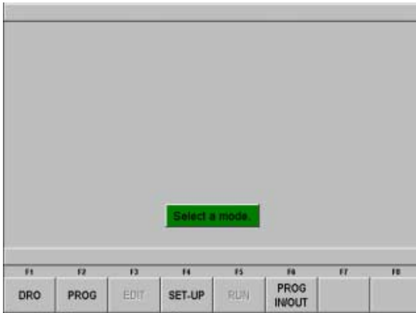
FIGURE 4.1.1 The main “select a mode” screen. Shown here, the Edit and Run Modes are grayed out because there is no program in current memory
