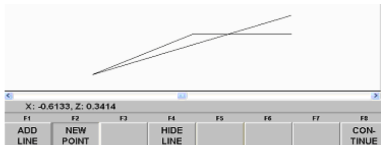
4.7.2.2 New Point allows you to end the new line anywhere on the drawing.
