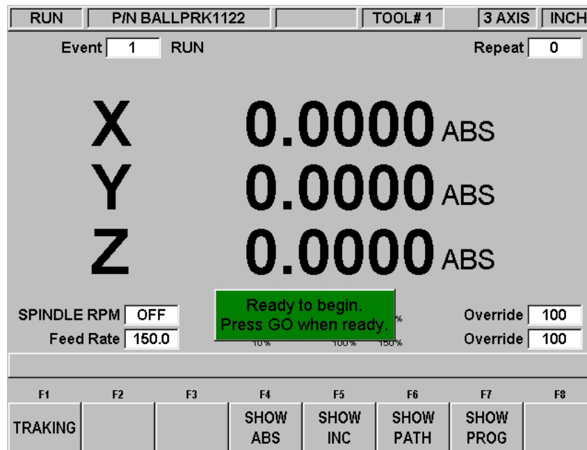
FIGURE 13.4 Press the GO feed key to start running.
