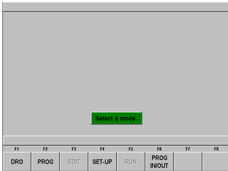
FIGURE 4.2.2 The main “select a mode” screen. Shown here, the Edit and Run Modes are grayed out because there is no program in current memory
