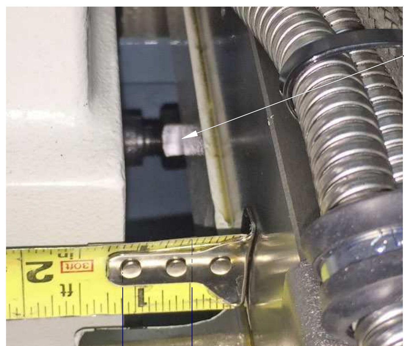
DETAIL K TAILSTOCK BUMPER 1" REQUIRED OFFSET
