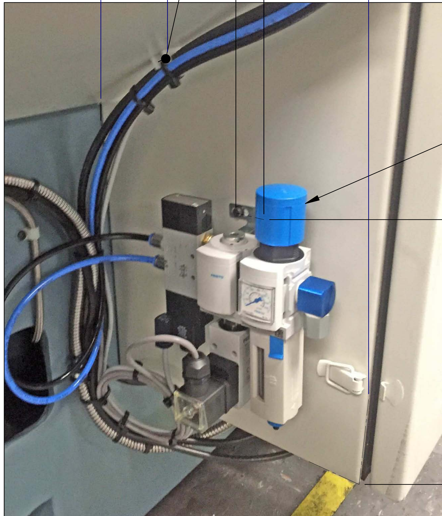
SECTION E-E AIR REGULATOR KIT (28622) INSTALLATION
