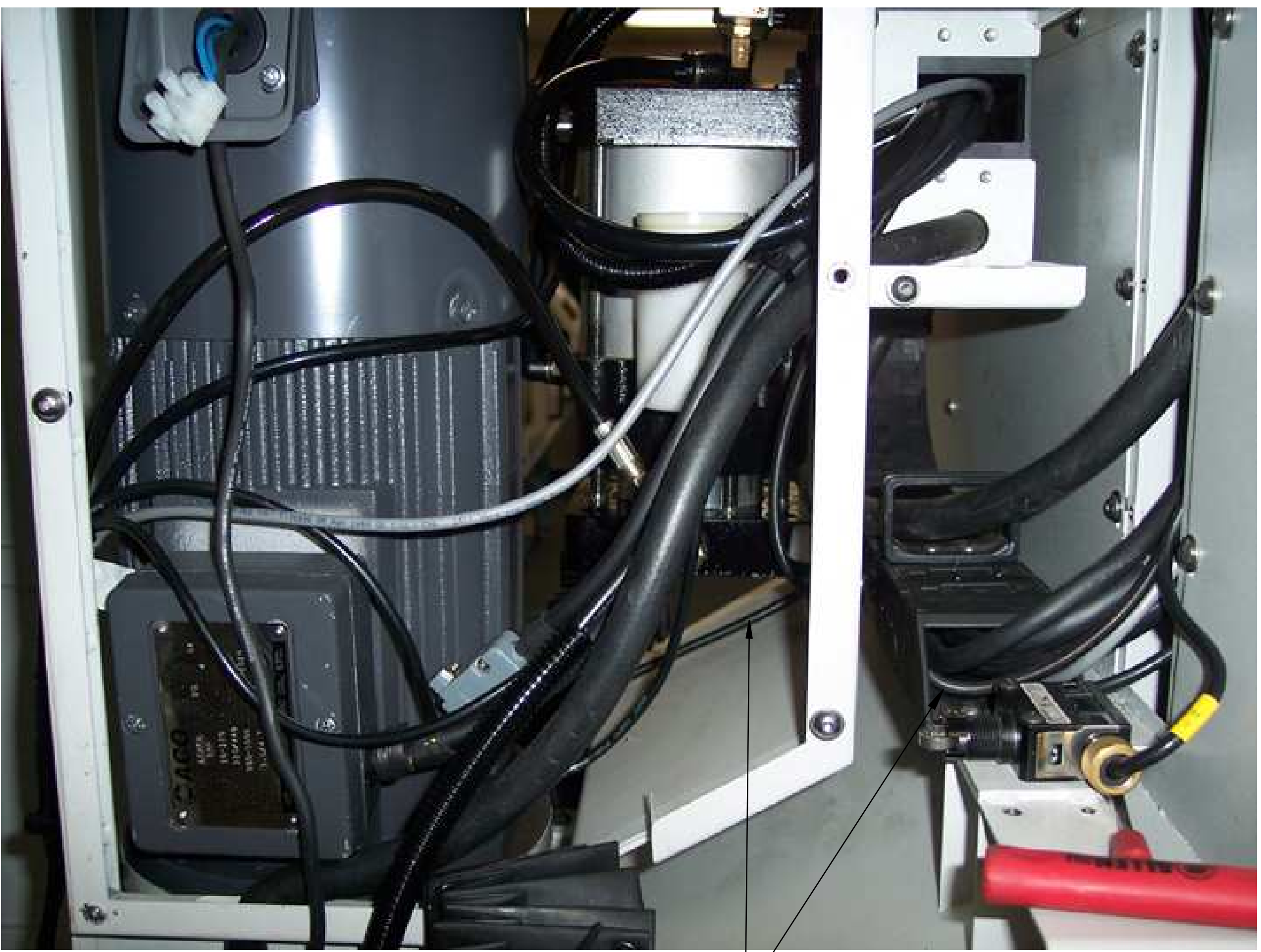
X AXIS LUBRICATION LINE COMING FROM THE MAIN DISTRIBUTION MANIFOLD TO THE X AXIS DISTRIBUTION MANIFOLD VIEWED FROM THE RIGHT SIDE OF THE SPINDLE.
