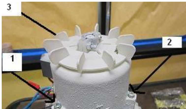
6. Remove Spindle Fan. Loosen and remove the 3 screws that secure it in place.
