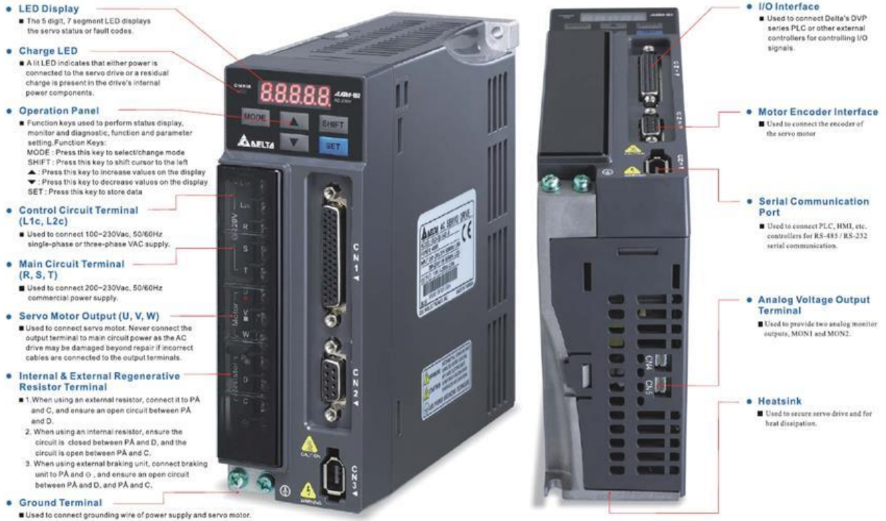
Figure 5.5.2b – Servo Drive Nomenclature
