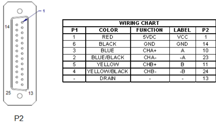
Figure 5.3c1 – EHW Port Pin Assignments
