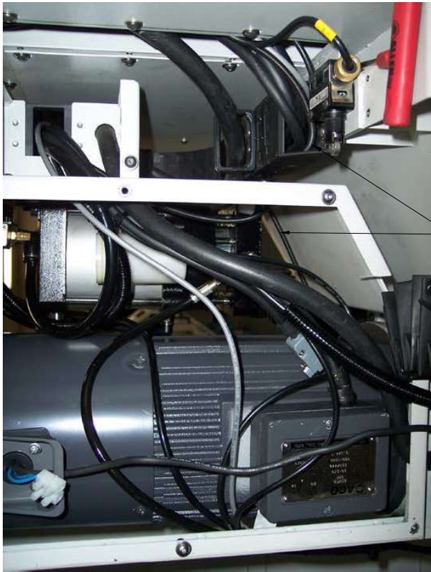
X AXIS LUBRICATION LINE COMING FROM THE MAIN DISTRIBUTION MANIFOLD TO THE X AXIS DISTRIBUTION MANIFOLD VIEWED FROM THE RIGHT SIDE OF THE SPINDLE.
