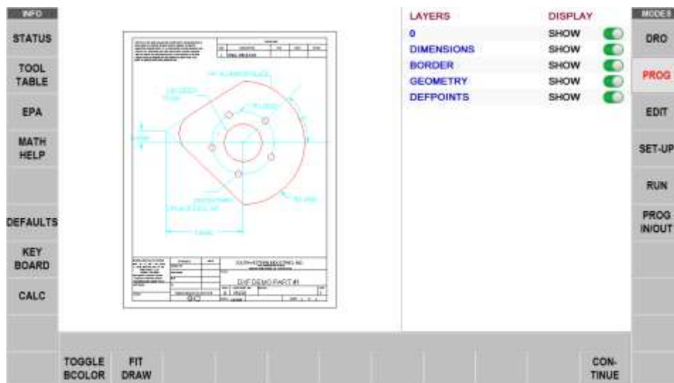
FIGURE 3.2.1 The first screen you see when the DXF Converter launches. Notice that the entire drawing, including borders and dimensions, is shown on this first view.
