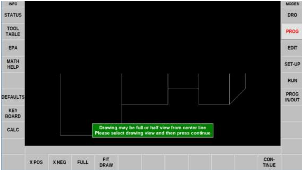
FIGURE 4.6.1 The X Pos key will display the portion of the drawing from the ABS 0 point you specified, down. This option is generally best.
