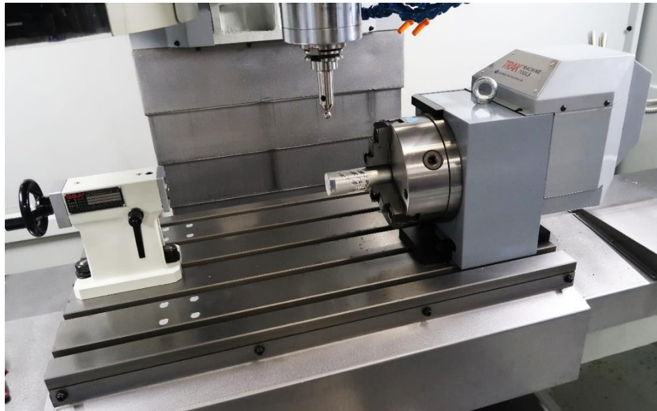
Figure 6.2a – 4 th Axis and Tailstock Option Mounted on TMC Table
