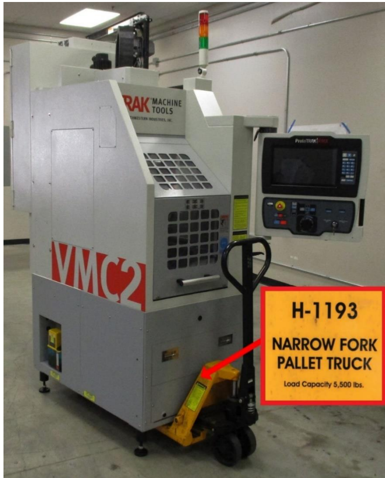
Figure 2.4b - Front Lift with 5,500 Capacity Pallet Jack
