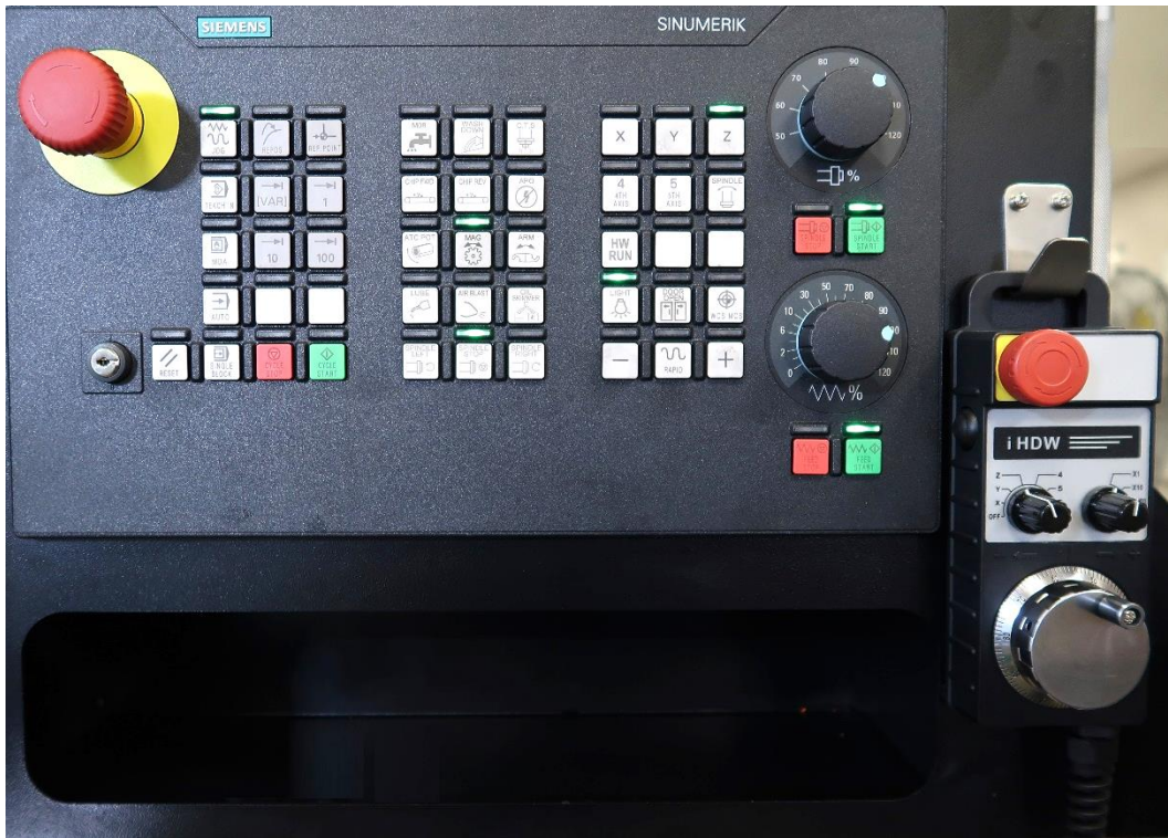
Figure 1.3.5.2 - VMCsi Password and Key Switch Access Levels
