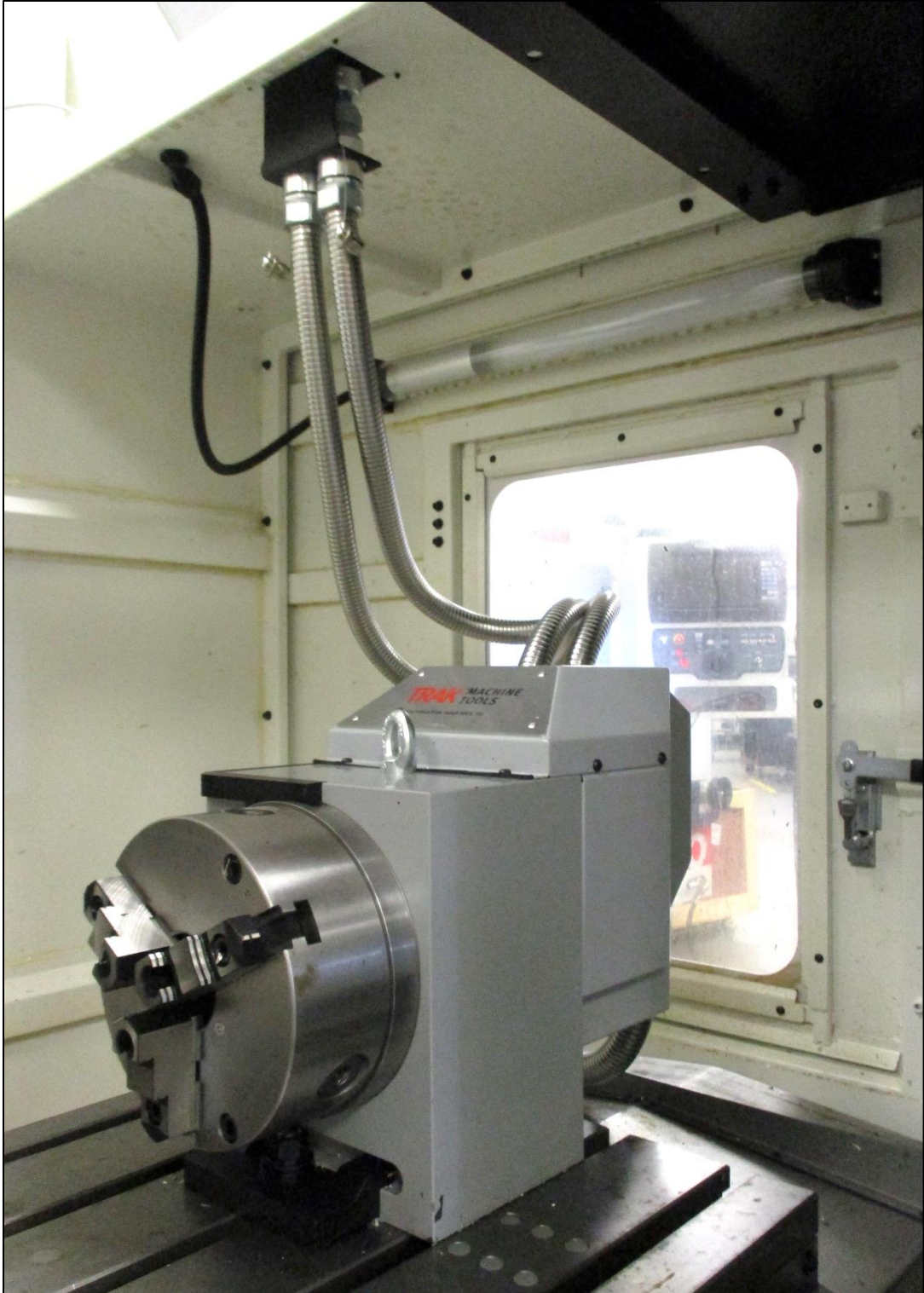
Figure 7.3c – 4 th Axis Option mounted on VMCsi showing cable routing
