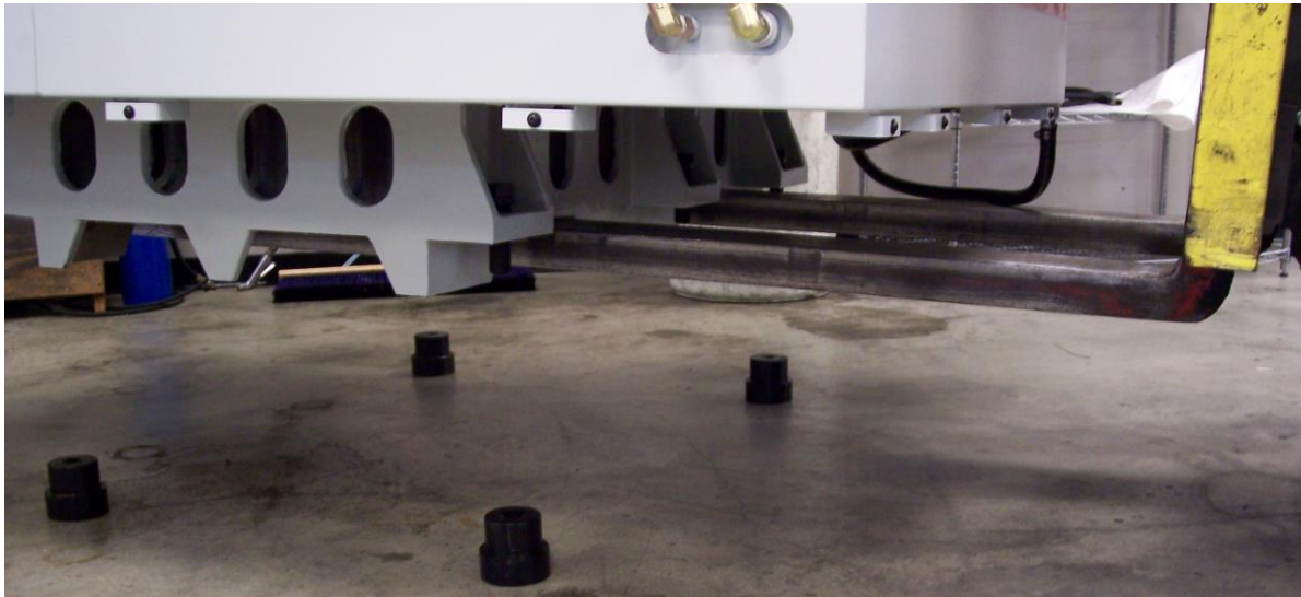
Figure 2.4b - Detail of Fork lift blades set in VMCsi base and proper set up of Leveling Pads
