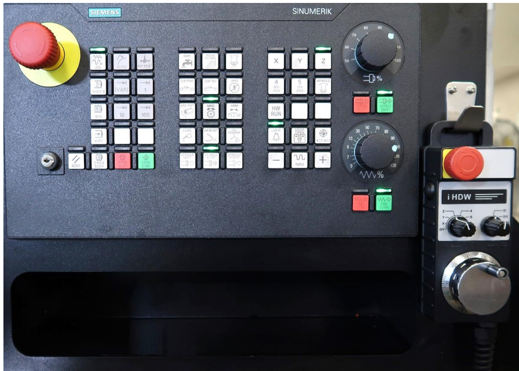
Figure 1.3.5.2 - VMCsi Password and Key Switch Access Levels
